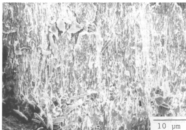
Figure 2 Secondary electron image showing aligned microstructure on cross section of fractured \text{Bi}_2\text{Sr}_2\text{Ca}_2\text{Cu}_3\text{O}_{10+y} tile made by the brush-on method.
